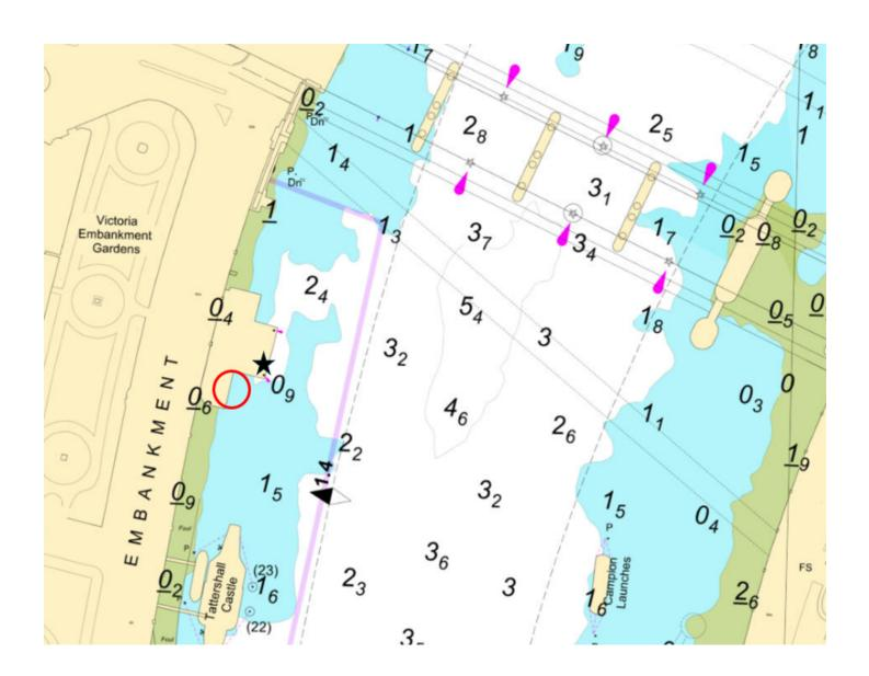
A set of warning lights are mounted vertically in front of a black backboard at the upper end of the site, near the CSO. The location of the light is shown on the chartlet (shown as a black star).
