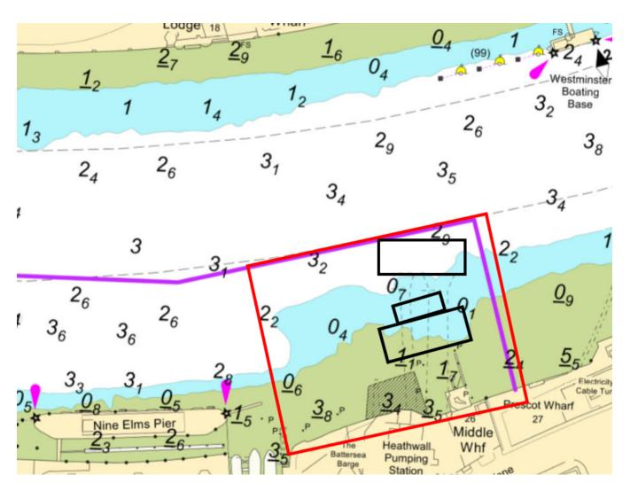
Works will involve the use of the TTT465 spudded barge with a long reach excavator and crawler crane, a muckaway and a supply barge. Safety boat **GUARD DOG** will be in attendance and maintain a listening watch on VHF channel 14.
